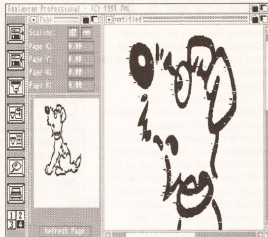
Handy Scanner isn't so handy at 400 dpi, covering the image in glitches which have to be removed by hand in zoom mode
